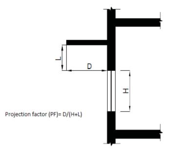
**Projection factor, side fin:** the ratio of the horizontal depth of the external shading projection to the distance from the window jamb to the farthest point of the external shading projection, in consistent units.
